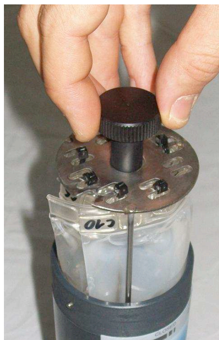
Pull up the fixing screw
