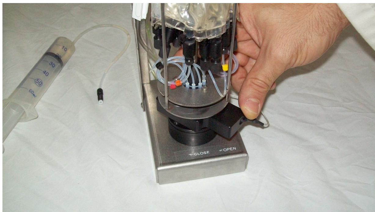
c) Open the reagent connector
